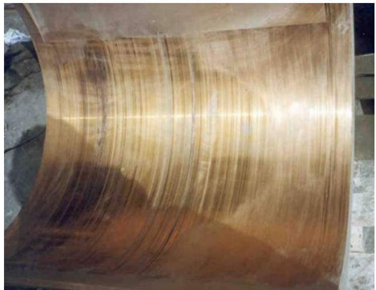
Figure C: Journal and bearing in boundary state due to inadequate film strength.
